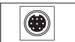
**Mini-DIN Serial Port:** Use this port to provide a direct terminal connection to a computer with a terminal emulation program. A serial cable (part number 73-1025) is included with the PDU. If you need to order a replacement cable, contact Tripp Lite Customer Support at [www.tripplite.com](http://www.tripplite.com).
