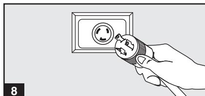
**9 Connect Equipment to PDU:** Do not exceed the load rating of the PDU. The total electrical current used by the PDU will be displayed on the digital meter in amperes.
