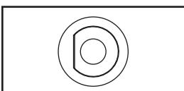
**Output Circuit Breakers (PDUMNH30):** Two circuit breakers (one per outlet bank) protect connected equipment against dangerous system overloads. If the total load on either of the PDU's outlet banks exceeds 20 amps, the associated circuit breaker will trip, cutting power to the entire outlet bank. Reduce the load on the outlet bank by unplugging some equipment; then press the circuit breaker in to restore power.
