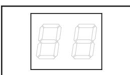
**Digital Load Meter (Ammeter, Models PDUMNH15 & PDUMNH20):** The total electrical current used by the PDU is displayed on the digital meter in amperes.
