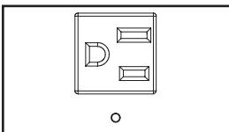
**NEMA 5-15R Outlets (Model PDUMNH15):** During normal operation, the outlets distribute AC power to connected equipment.
