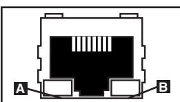
**Ethernet Port:** Use this RJ-45 jack to connect the PDU to the network with a standard Ethernet patch cable. The Link LED **A** and Status LED **B** indicate several operating conditions, as shown in the table below.
