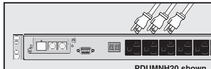
**10 Cord Retention (Optional):** If you attached the cord retention shelves, use them to secure equipment power cords. Attach each cord to the retention shelf by looping the cord and securing it to an attachment point with one of the included cable ties. Make sure that each equipment power cord can be unplugged from the PDU without removing the cable tie.
