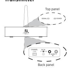
**SIGNAL** indicator lights green when the audio is present and the transmitter is broadcasting
