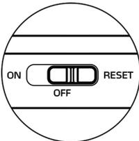
A circular diagram of a 3-way power switch. The switch is a horizontal slider with three positions: 'ON' on the left, 'OFF' in the center, and 'RESET' on the right. The slider is currently in the 'OFF' position. | <h3>3-Way Switch</h3> <ul style="list-style-type: none"><li>• Slide to the left to turn the receiver on.</li><li>• Slide to the center position to turn the receiver off.</li><li>• Slide to the right to reset the receiver.</li></ul> |
