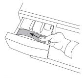
The card will then bend slightly and you can easily remove it. To fit the card, bend it slightly in order to easily insert it into the holder in the detergent compartment.
