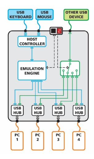
FIGURE A-1. EMULATED AND ENUMERATED SWITCHING
