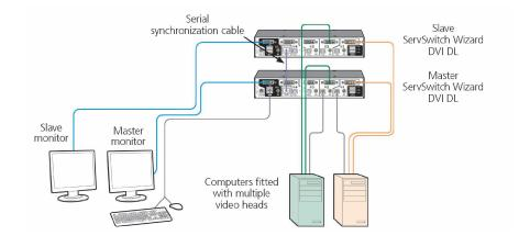
FIGURE 3-17. SYNCHRONIZING MULTIPLE UNITS
