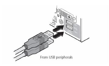
FIGURE 3-3. CONNECTING USB PERIPHERALS TO THE USER CONSOLE
