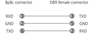
Serial remote control and flash upgrade cable (10p10c)
