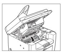
Close the printer cover and lower the scanning platform.
