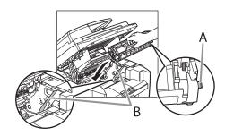
Push the toner cartridge to make sure it is properly set in the machine.
