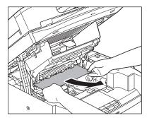
Gently pull the jammed paper between the fixing assembly (A) and transfer roller (B) until the leading edge emerges from the machine.
