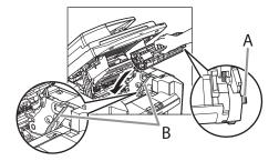
**9** Push the toner cartridge to make sure it is properly set in the machine.
