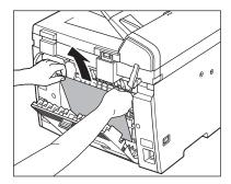
If the jammed paper is badly folded, similar to the folds of an accordion, ease the jammed paper loose and then pull it out from the machine.
