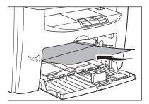
When setting an envelope, gently insert the envelope into the multi-purpose tray with the print side up and the right edge (i.e., closer to the stamp) first.
