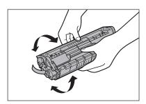
Place the toner cartridge on a flat surface and pull the seal completely out.
