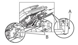
Push down the toner cartridge to make sure it is properly set in the machine.
