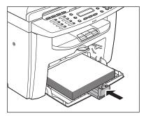
Aligning the protrusions (A) on the both sides of the dust cover to the guides (B) inside the machine, set the dust cover.
