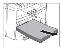
Remove the paper cassette by lifting up the front-end of the paper cassette and pulling it forward.
