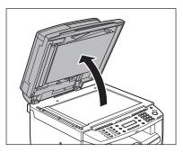
2 Clean the platen glass and the underside of the ADF with a cloth dampened with water. Then, wipe the area with a soft, dry cloth.
