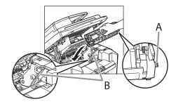
Push the toner cartridge to make sure it is properly set in the machine.
