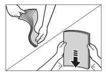
Load the paper into the paper cassette with the print side up. Make sure the paper stack sits below the small fin (A) on the side paper guide.
