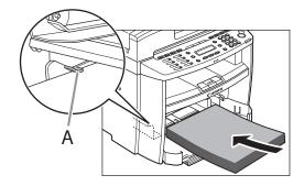
Adjust the paper guide rail to match the size of paper.
