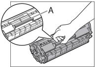
Insert the toner cartridge so that the protrusion (A) on the right side of the toner cartridge fits into the guide (B) located on the right side of the machine and slide it down parallel to the guide.
