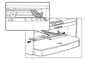
When setting paper, gently insert the paper into the multi-purpose tray with the print side up.
