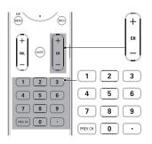
Press **CHANNEL +/-** on the side of the TV. For digital channels, press a number (1 to 135) followed by a dot ":" and then the corresponding sub channel number (1 to 135). Ex. 108.30.
