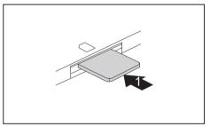
► Insert the SIM card into the slot so that the chip is facing downwards and the angled corner is at the front left, facing towards the slot (1). Ensure that you hear the SIM card click into place.
