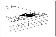
► Insert the hard disk into the hard disk compartment in the direction of the arrow (1) .
