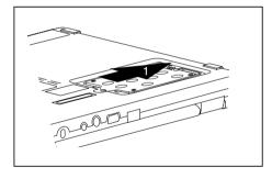
Use the pulling aid to pull the hard disk out of the bay in the direction of the arrow (1).
