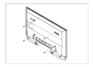
4. Remove safety pin (3) and insert the 4 product holders into the corresponding bracket holes (1). Then place the product(2) so that it is firmly fixed to the bracket. Make sure to re-insert and tighten the safety pin (3) to securely hold the product to the bracket.
