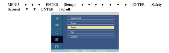
This function prevents after-images on the screen by moving all the pixels on the LCD according to a pattern.
