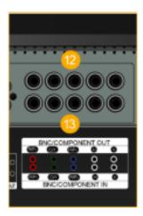
12 BNC/COMPONENT OUT[R/PR, G/Y, B/PB, H, V]
