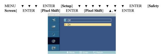
To prevent after-images on the screen you can use this function, so that every minute pixels on the LCD are moved in horizontal or vertical direction.
