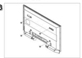
Tighten the 4 screws in step 2 (plastic hanger + screw **B**)to the rear holes of the product.
