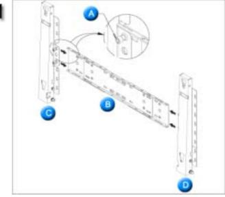
Insert and tighten the Captive Screw in the direction of the arrow.
