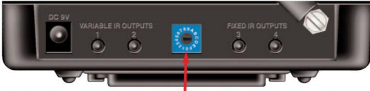
Check that the arrow pointer in the center of the wheel is pointed to 0, the default “interference sniffing” position. If it is not, use a small flat blade screwdriver (included) to set the RF ID# to 0.
