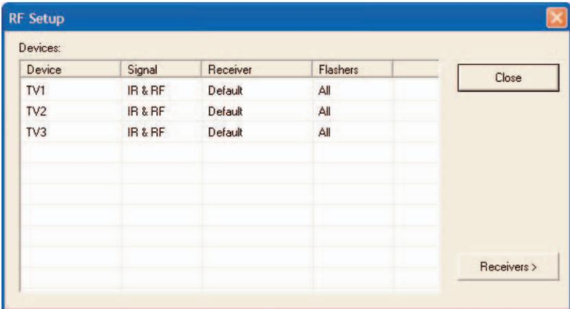
By looking at the Signal column, you can see that the factory default programming sets all of the devices to send both IR and RF commands. If you look at the column for Flashers, you can see that the default sends IR commands for all devices to ALL of the flashers. Both options must be changed for identical components. Additionally, you must disable the Front Blaster (see page 6 for directions).
