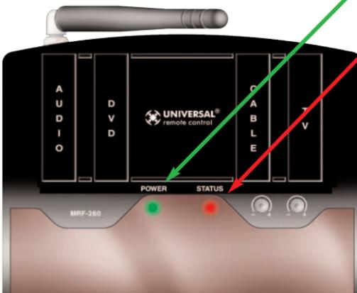
The green POWER LED indicates that the MRF-260 is powered on.
