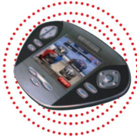
2. The MRF-260’s integrated Narrow Band RF receiver receives commands from any Narrow Band remote control.
