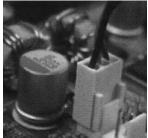
4. Connect the attached power connection to an available TX3 connector.
