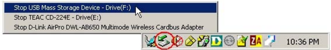
Figure 27. Click the Unplug or Eject Hardware icon, then select the Migo-enabled device (it will be referenced as a USB mass storage device) from the pop-up menu.
