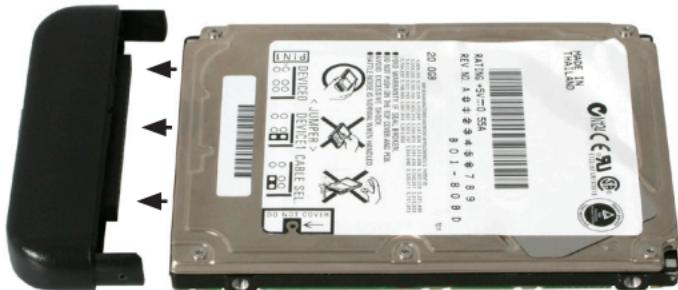
4. Insert the top panel and attached hard drive into the bottom panel.
