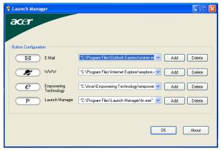
Launch Manager allows you to set the four easy-launch buttons located above the keyboard. **"Easy-launch buttons" on page 18** for the location of the easy-launch buttons.
