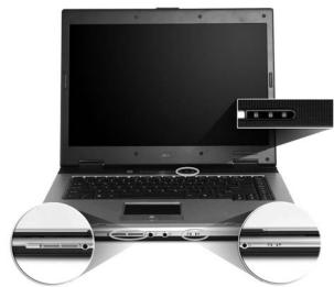
The power, battery and wireless communication status indicators are visible even when the LCD display is closed.
