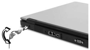
Wrap the computer security lock cable around an immovable object such as a table or handle of a locked drawer. Insert the lock into the notch and turn the key to secure the lock. Some keyless models are also available.
