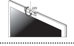
**Note:** DO NOT rotate the camera clockwise to prevent damage to the device.
