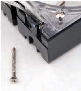
3. Use the long screws provided to secure the fan to the mount.
