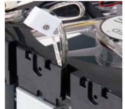
5. Clip the fan mount/fan assembly onto the back of an empty HDD cage.
