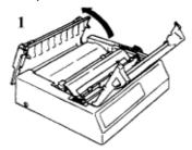
Turn the platen knob to back the paper all the way out, and remove any torn pieces of paper.
