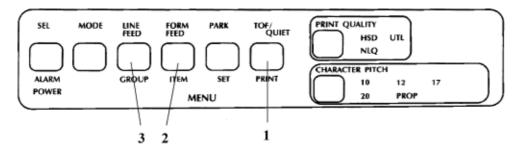
Make sure the printer is deselected. Hold down the **TOF/QUIET** button and press: **FORM FEED** to move the paper up, or **LINE FEED** to move the paper down.
