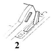
To return continuous forms to the printer, make sure the paper lever is set for continuous forms (3).
