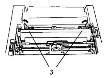
Pull the paper through the opening between the printer and the rear cover and place the first two sprocket holes on each side of the page over the pins (4).
