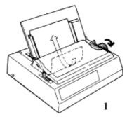
Pull the bail lever forward to load in a fresh sheet of paper (2).
