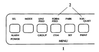
To activate this feature, press the **MODE** button and use the **GROUP**, **ITEM** and **SET** buttons to change the FORM TEAR OFF setting to 500 ms (1). (See Chapter 5 ( ) for details on how to use the menu). Press the **MODE** button to exit the Menu mode, then use the **TOF/QUIET** and **FORM FEED** or **LINE FEED** buttons to set the top of form as described above (2).
