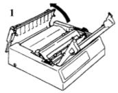
Fold some continuous-feed paper over three times to produce a page four sheets thick and load it onto the tractors.
