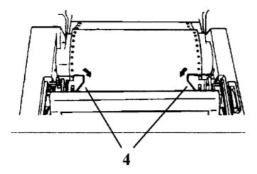
Close the rear cover (make sure the paper separator is flat on the printer), open the guide wire, and close the access cover (5).
