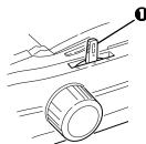
5 Adjust the paper guides (1) for the size paper you are using, then place a sheet of paper in the sheet guide.
