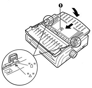
12 Place the wire guide ("1" in the illustration for the step above) in the sheet guide on the pull-up roller assembly.
