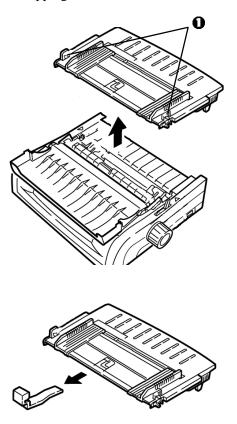
5 Reinstall the sheet guide: insert the clips on either side of the separator into the notches marked with a triangle, then press down to secure the separator in place.
