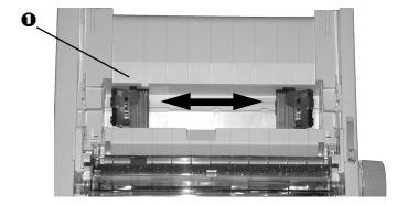
7 Open the tractor covers and place continuous forms paper on the first two pins of either tractor, then close the *left* tractor cover.
