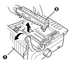
**4** Lift the sheet guide (1) and reload paper. Make sure you lock the tractor covers.
