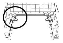
11 Lower the sheet guide and slide it toward the front of the printer until the marks align.
