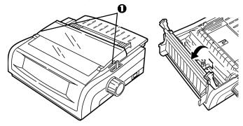
2 Remove the printhead shipping restraint.
