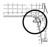
**10** Adjust the left tractor until the holes in the paper are centered on the pins then lock the lever and close the left tractor cover.
