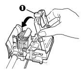
**4** Turn the take-up knob (1) in the direction of the molded-in arrow to take up any ribbon slack.
