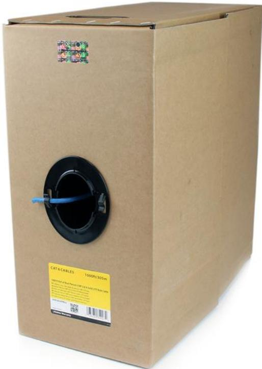
This Cat6 500MHz Solid UTP Cable is CMR rated for use in walls, conduit, ceilings, etc. and is packaged as a 1000ft bulk roll. The cable features a blue PVC jacket that provides both flexibility and durability, while making it easier to color code network cable connections.
