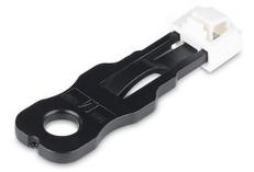
Install these 10 RJ45 Port Locks into standard RJ45 (modular 8P8C) jacks/Ethernet LAN ports to restrict access and to protect against physical damage, dust, and contaminants.
