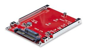
Convert and connect a PCIe M.2 NVMe/AHCI SSD to a 2.5inch form factor to install in a U.3 drive bay or backplane.
