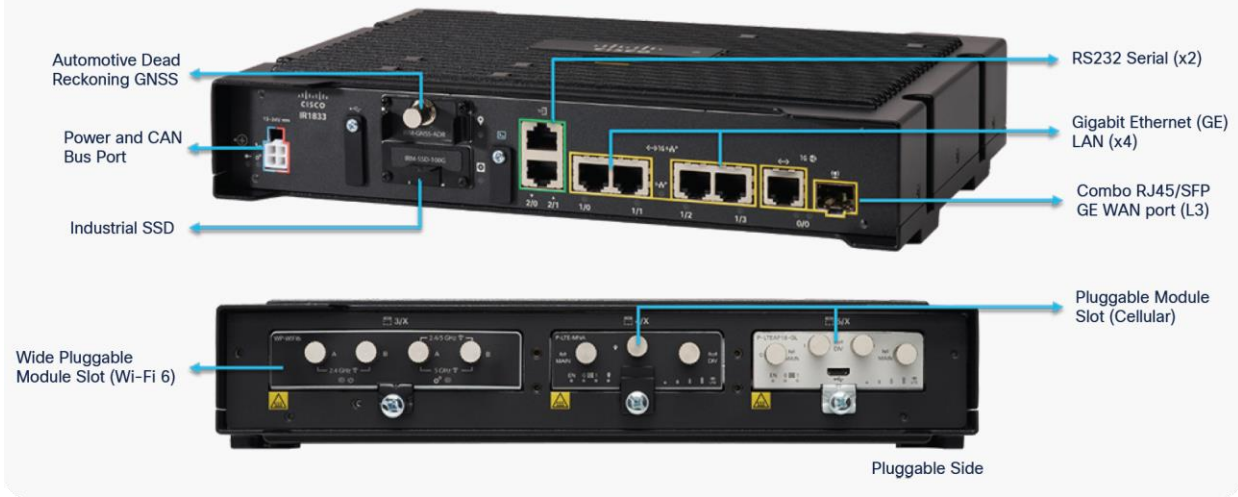
Figure 5. IR1833-K9 interface ports
