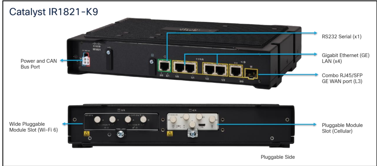
Figure 3. IR1821-K9 interface ports
