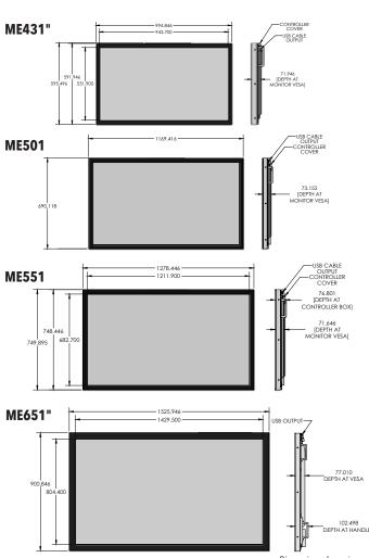
Dimensions shown in mm Projected Capacitive Touch Screen Overlay Patent Pending
