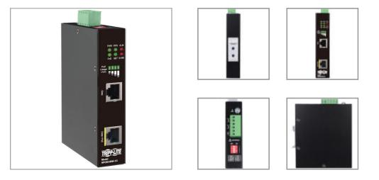
Industrial-grade PoE+ injector uses existing Cat6 cable to supply 90W power + data up to 328 ft. to a PoE device connected to a non-PoE switch.
