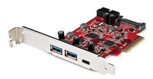
This 5-port USB 3.2 Gen 2 (10Gbps) combo card makes it easy to add to the performance and connectivity of your computer. The USB 3.2 card offers a USB Type-C port (10Gbps), two traditional USB Type-A ports (10Gbps), and a motherboard header (USB 5Gbps).
