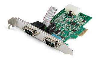
This multiport PCI Express RS232 serial adapter card lets you add two RS232 (DB9) serial ports to your computer through a PCI Express (PCIe) slot, as if they were native serial ports. The dual port PCIe serial card enables you to interact with serial devices, such as card readers, printers, PIN pads, and modems, at speeds of up to 921.6Kbps.
