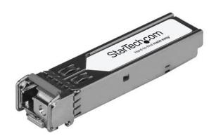
The SFPGE10KT5R3 is a Juniper SFPP-10GE-LR compatible fiber transceiver module that has been designed, programmed and tested to work with Juniper brand switches and routers. It delivers dependable 1 GbE connectivity over fiber cable, for 1000Base-BX10-D compliant networks, with a maximum distance of up to 40 km (24.8 mi).
