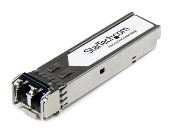
The JD094A-ST is an HP JD094A compatible fiber transceiver module that has been designed, programmed and tested to work with HP brand switches and routers. It delivers dependable 10 GbE connectivity over fiber cable, for 10GBase-LR compliant networks, with a maximum distance of up to 10 km (6.2 mi).
