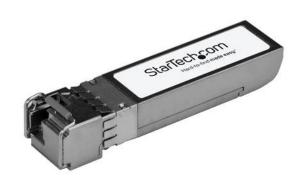
The J9151A-BX-D-ST is an HP J9151A-BX-D compatible downstream fiber SFP+ transceiver which pairs with StarTech.com's J9151A-BX-U-ST. They are designed, programmed and tested to work with 10GBase-BX compatible MSA switches and routers. The SFP+ transceiver module supports a maximum distance of up to 10 km (6.2 mi) and delivers dependable 10 GbE connectivity over fiber cabling.
