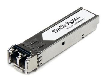
The EW3Z0000585-ST is a Citrix EW3Z0000585 compatible fiber transceiver module that has been designed, programmed and tested to work with Citrix brand switches and routers. It delivers dependable 10 GbE connectivity over fiber cable, for 10GBase-SR compliant networks, with a maximum distance of up to 300 m (984 ft).
