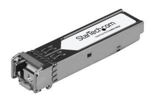
The 10057H-ST is an Extreme Networks 10057H compatible upstream fiber SFP transceiver which pairs with StarTech.com's 10056H-ST. They are designed, programmed and tested to work with 1000Base-BX-U compatible Extreme Networks switches and routers. The SFP transceiver module supports a maximum distance of up to 10 km (6.2 mi) and delivers dependable 1 GbE connectivity over fiber cabling.
