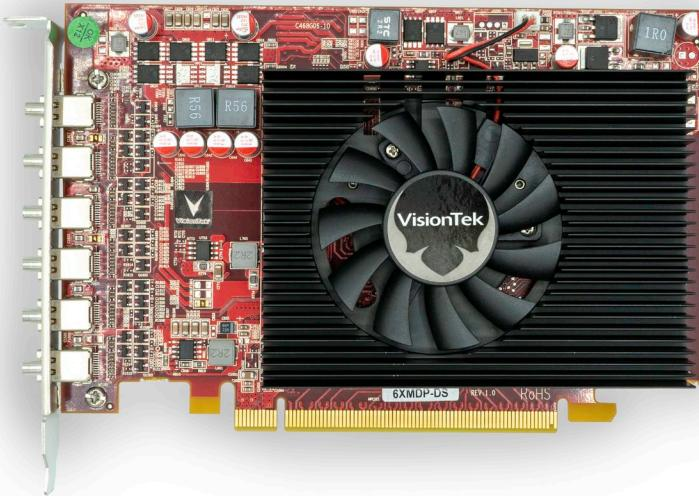
The VisionTek Radeon 7800M offers advanced video and display technologies, as well as support for DirectX 11 for the most versatile solution for digital signage. Designed for full sized systems, you can make use of amazing multimedia capabilities utilizing AMD ZeroCore Power Technology. The 7800M also offers more workspace by supporting up to six monitors.
