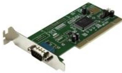
This 16550 Serial PCI Card can be installed in a computer PCI slot to add an RS232 serial port - a cost-effective solution for connecting any new serial device or old legacy serial device, with data transfer rates of up to 115.2 Kbps. The serial card features a low profile/half-height bracket, suitable for installation in low profile/small form factor computer cases.
