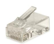
The WBOX Standard CAT5E modular plugs are designed for RJ45 connector installations. Designed for the conductors to be arranged in a high low stagger for high performance. The 2 pronged contacts provide reliable connections with solid and stranded wire.
