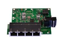
Embedded format, takes up minimal space, with mounting holes are connected to Functional Earth
