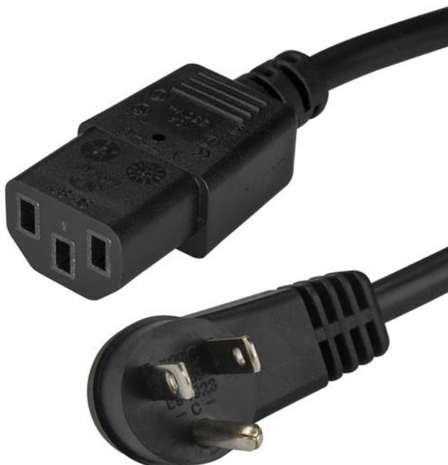
This NEMA 5-15P to C13 power cord features a right-angled plug, which positions the connector in such a way that it does not block other available outlets. The cable is especially useful when plugging into a dual AC wall outlet as it frees up the second outlet for another power cord.
