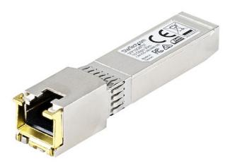
The SFP10GBTST is an MSA compliant copper SFP transceiver that's designed, programmed and tested to work with 10GBASE-T compatible switchess and routers. The SFP+ transceiver module supports a maximum distance of up to 30 m (98.4 ft.) and delivers dependable 10 GbE connectivity over copper cabling, which is a cost-effective alternative to fiber-optic cable setups. <br/>
