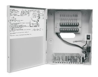
The 0E-1275AD9 is a cost effective way to power up to 9 cameras in a security system. Individual class PTC fuses for each output as well as over current voltage protection that provides a high level of protection.
