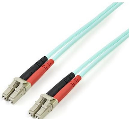
This fiber optic cable lets you connect 40GBase-SR4, 100GBase-SR10, SFP+ and QSFP+ transceivers in 40 and 100 Gigabit networks. The OM4 cable supports Vertical Cavity Surface Emitting Laser (VCSEL) and LED light sources and is backward compatible with your existing 50/125 equipment.
