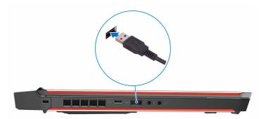
**6** Connect a USB Type-C to Type-A dongle to the USB 3.0 (Type-C) port at the left side of your computer.
