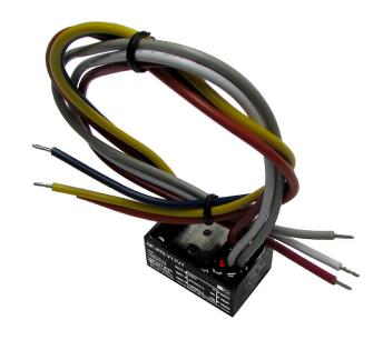
OE-FRLY12V7 is an encapsulated multi-voltage relay suited to applications requiring a remote relay for control or status feedback. It includes long flying leads selectable for the input control voltage to be applied. A red LED indicates relay coil is energized. Applications include Fire Alarm Control, security systems, HVAC, temperature control, lighting systems and energy management. OE-FRLY12V7 is UL 864 listed for Fire Alarm Control Equipment. Includes mnting./wiring hardware.
