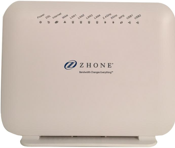
6768-W1 is a most versatile Broadband gateway for service providers that are seeking a single hardware that can support ultra-high bandwidth applications using VDSL2 technology, Gigabit Ethernet for FTTx. Using VDSL2 mode, the 6768-W1 series can support downstream connection rate at 100Mbps and 50Mbps upstream for triple play applications, or just double the bandwidth for existing ADSL2+ customers.
