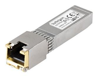
The GLCTSTTAA is a TAA compliant Cisco GLC-T compatible copper transceiver module that has been designed, programmed and tested to work with Cisco brand switches and routers. It delivers dependable 1 GbE connectivity over copper cable, for 1000BASE-T compliant networks, with a maximum distance of up to 100 m (328 ft).
