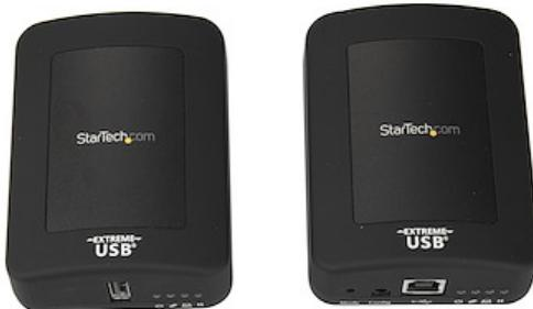
This single-port USB 2.0 extender lets you access and use your USB device up to 100 m away over Cat5e or Cat6 cable. And, because it can be powered by either the local or the remote unit, you have more flexibility to place your USB device exactly where you need it. It's the perfect USB extension solution for warehouses, factories, classrooms, boardrooms, homes, or offices.
