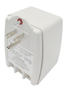
The OE-PPS2450 is a plug-in 24VAC, 50VA plug-in transformer that provides reliable AC power for a wide variety of indoor security and surveillance products and applications. It is auto-resetting PTC fuse protected and includes a power indicator LED. Grounding is provided via a third screw terminal and ground plug. Complies with DOE Level VI Efficiency requirements for alarm industry plug-in power supplies.
