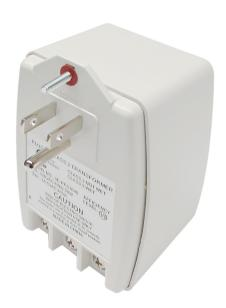
The OE-PPS1650 is a plug-in 16.5VAC, 50VA plug-in transformer that provides reliable AC power for a wide variety of indoor security and surveillance products and applications. It is auto-resetting PTC fuse protected and includes a power indicator LED. Grounding is provided via a third screw terminal and ground plug. Complies with DOE Level VI Efficiency requirements for alarm industry plug-in power supplies.
