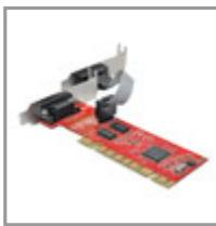
Adds 2 DB9 serial ports to your PCI computer or server or replaces existing DB9 ports. Low-profile bracket is designed for shorter computer cases.
