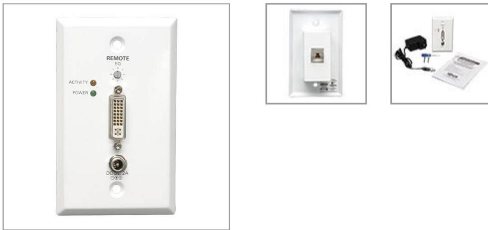
Receiver wallplate extends a DVI-D single-link signal via one Cat5e/6 patch cable up to 200 ft. with a Tripp Lite B140-002 or B140-004 extender/splitter transmitter unit (sold separately).
